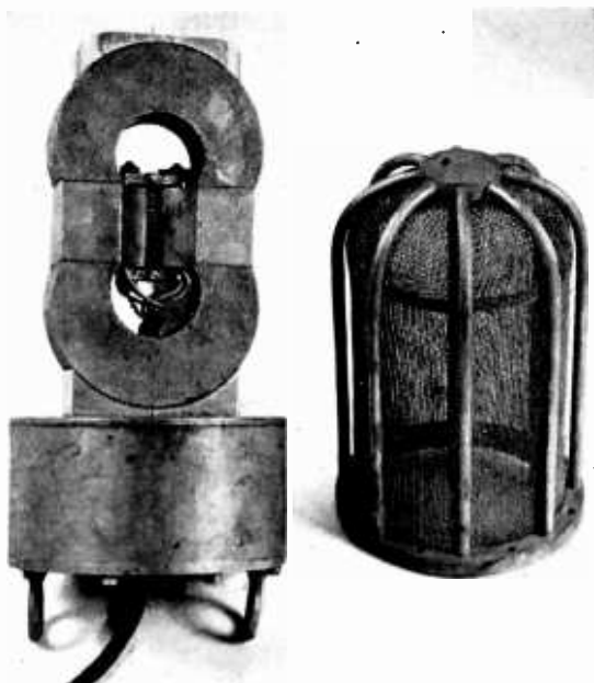
Fig. 11—Subaqueous velocity microphone with the protective screen removed.
