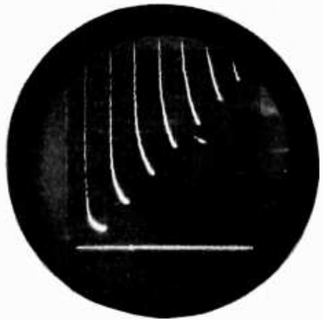
Fig. 7—Phosphorescence build-up of P7 yellow, using B_1 to B_7 pulsed excitation (blue light).
