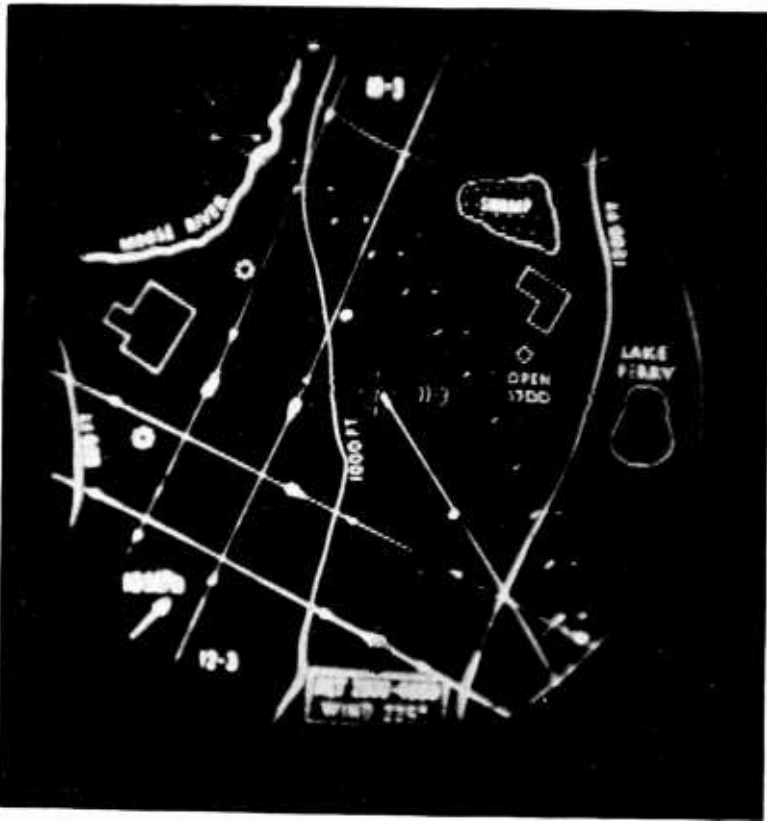
Fig. 9—PPI information and optically superimposed aerial map simultaneously picked-up by a Storage Crthicon.
