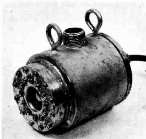
Fig. 19—High frequency dynamic subaqueous loud speaker.
